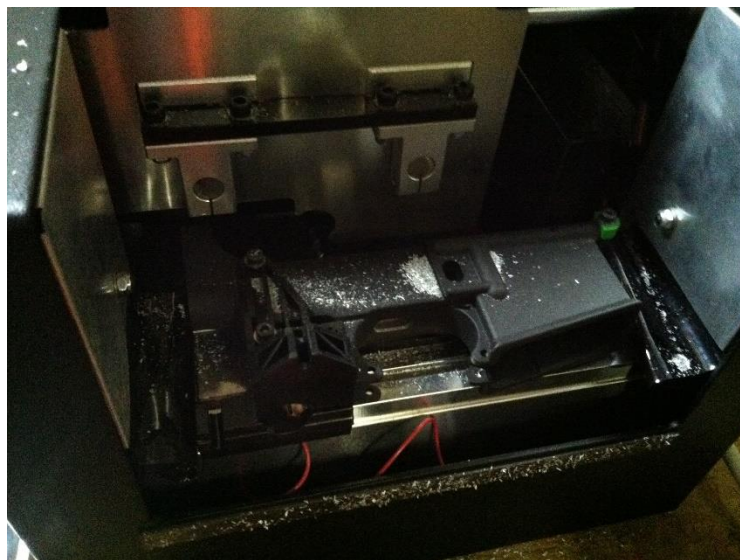
Figure 42: Chip guard removed, not vacuumed
