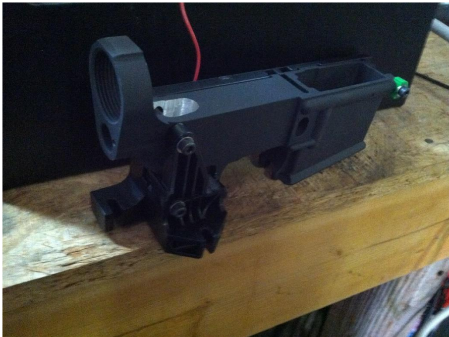
Figure 28: Lower with all installed jigs (left, right and front)
