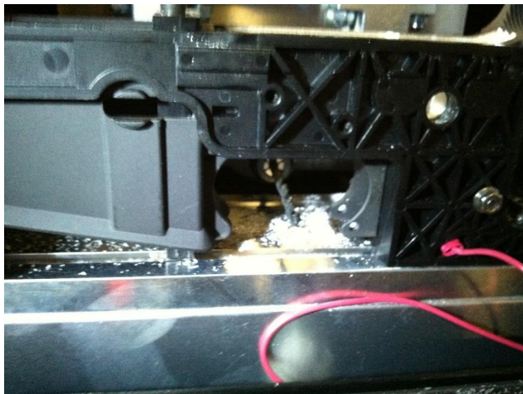
Figure 59: Spindle in proper position to insert drill bit.
