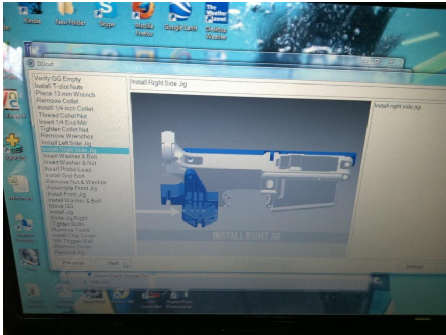
Figure 19: dd File illustration of installed right hand jig.
