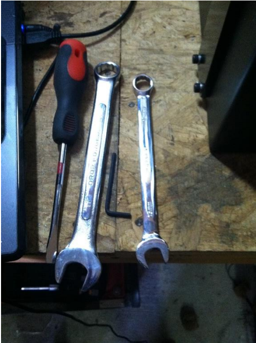
Figure 8: Needed tools, 13, 17mm wrenches, 3mm Allen wrench and flat blade screw driver
