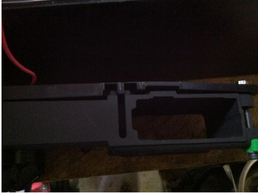
Figure 17: Improperly seated left hand jig, note bowing in center
