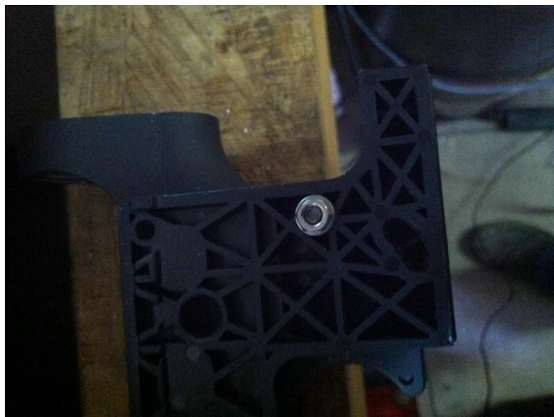
Figure 22: Properly installed 4x45 bolt, nut and washers.
