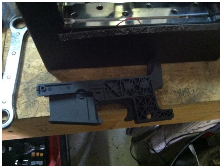
Figure 16: Properly installed left hand jig
