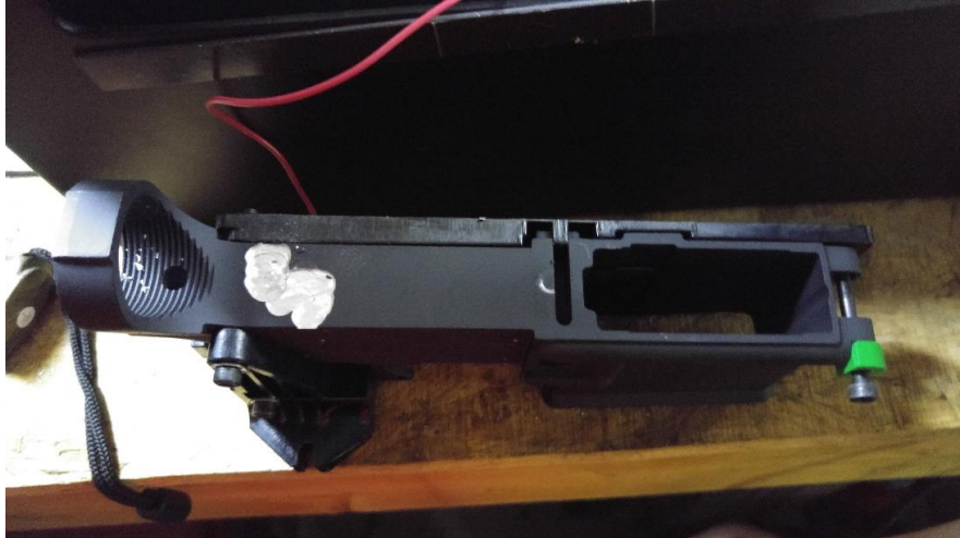
Figure 39: Result of attempting to machine a 78% lower (no rear takedown lug slot)
