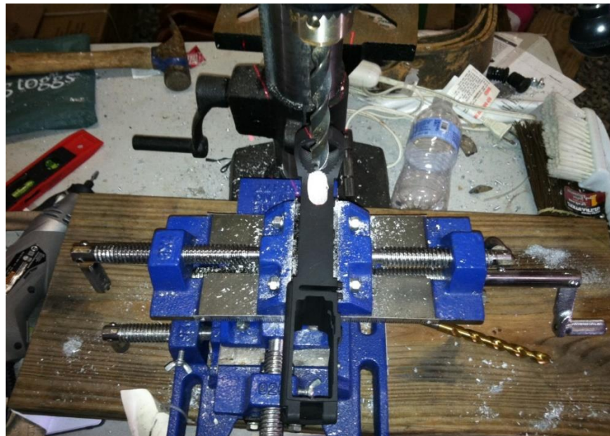
Figure 3: 78% Lower after being milled for the rear takedown slot.
