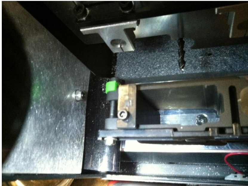
Figure 51: Magazine well jig and T-slot bolt in place. Note nut and washer in place on forward takedown lug bolt.
