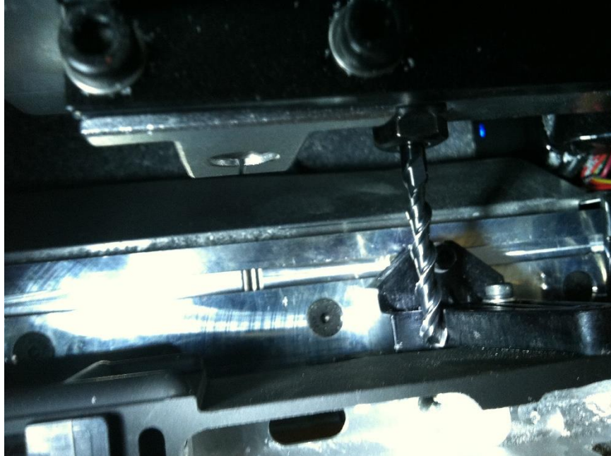
Figure 54: End mill is down and to the right nestled into the corner of the right hand jig face.
