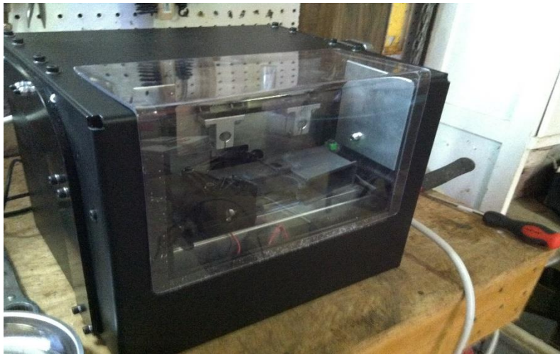
Figure 36: Properly installed chip guard.
