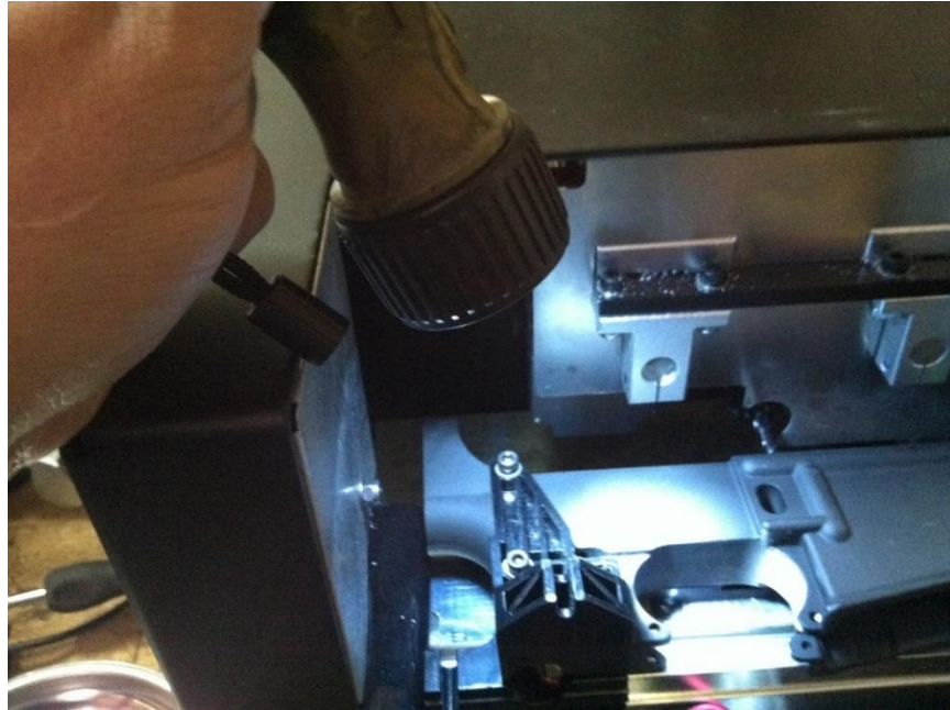
Figure 31: Using a small flashlight can help with bolt hole alignment with the T-slot nuts.
